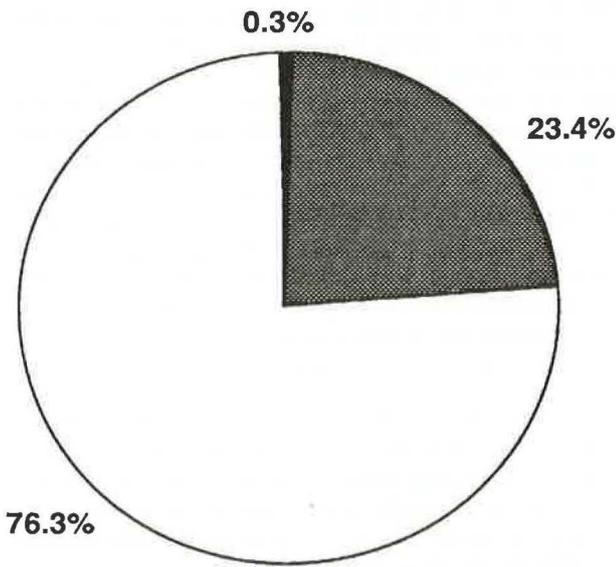
Fig. 3. - Distribution of the oxygen concentrators (OCs) related to  $F_{O_2}$  supply (OCs out of order ■ : measured  $F_{O_2} < 50\%$  (n=7); OCs not in optimal order, ▨ :  $50\% \leq$  measured  $F_{O_2} <$  predicted  $F_{O_2}$  (n=565); OCs in good working order □ : measured  $F_{O_2} \geq$  predicted  $F_{O_2}$  (n=1,842).  $F_{O_2}$ : oxygen fraction.
