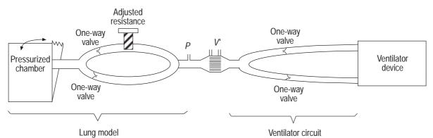
Fig. 1. – The lung model consisted of a pressurized chamber connected to a circuit comprising an expiratory line and an inspiratory line with adjustable resistance. the compliance of the chamber was set at 30 mL·cmH<sub>2</sub>O<sup>-1</sup>. A pneumotachograph (flow (V')) and a differential pressure transducer (pressure (P)) were inserted between the chamber and the circuit of the lung model.
