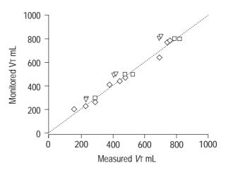
Fig. 3. – Relationship between the observed VT and the monitored VT for the three ventilators providing VT monitoring ( $\Box$ : O'nyx plus;  $\diamond$ : Ecole-3-XL;  $\nabla$ : Monnal DCC).
