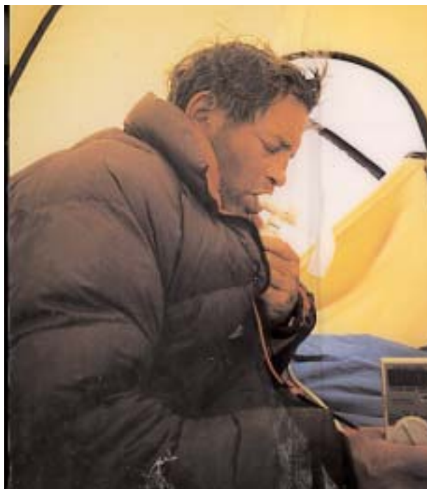
Fig. 1. – Measurement of alveolar partial pressure of oxygen on the South Col of Everest (8,000 m). The subject is exhaling into a tube connected to an oxygen fuel cell, which delivers a voltage proportional to the partial pressure of oxygen. Its output was measured in millivolts using a portable battery-operated digital voltmeter.
