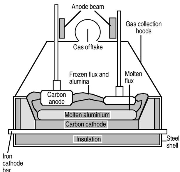
Fig. 2. — Aluminium smelter reduction cell with prebaked anodes (prebake cell) printed with permission [16].
