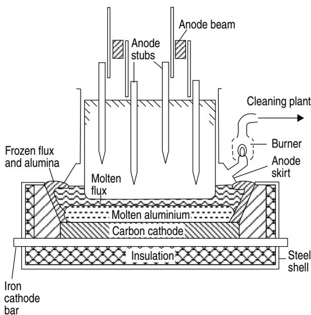
Fig. 1. — Aluminium smelter reduction with anodes baked on the spot (Söderberg cell) printed with permission [16].
