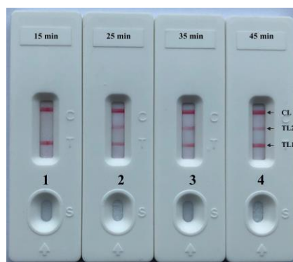
Figure S6. The optimal duration of time required for COVID-19 RT-MCDA-BS assay Four reaction times ( A , 15 min; B , 25 min; C , 35 min; and D , 45 min) were tested and compared at 64 °C. COVID-19 RT-MCDA reactions were conducted using the LoD level of templates ( 5 \times 10^0 copies of each of F1ab-plasmid and N-plasmid), and the templates at the LoD level could be detected when the RT-MCDA reaction only lasted for 25 min ( Biosensor 2 ).
