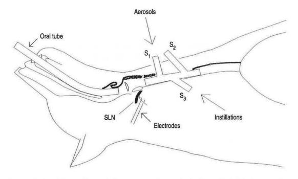
Fig. 1. – Experimental set-up. When aerosols were administered, the upper airway was functionally isolated by inflating the cuff of a Foley catheter, introduced through  $S_3$ , between  $S_1$  and  $S_2$ . See text for further details. SLN: superior laryngeal nerve.
