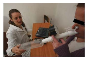
**FIGURE 1.** Sampling of exhaled breath for smellprint analysis by electronic nose. The subject inhales though a volatile organic compound filter and exhales with stable flow rate against resistance.
