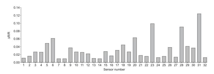
FIGURE 3. A representative smellprint of volatile organic compounds in exhaled breath recorded by an electronic nose with 32 polymer sensors as the change in sensor resistance (ΔR/R). The exhaled breath was collected from a lung cancer patient.
