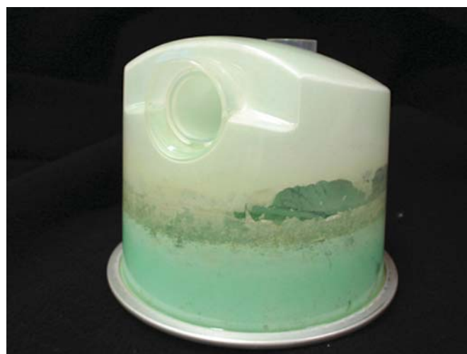
FIGURE 1. A continuous positive airway pressure humidifier chamber coated with a green residue due to a build up of calcium stearate.
