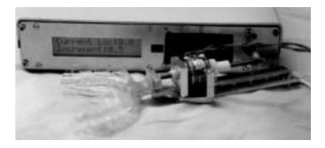
FIGURE 1. A remotely controlled mandibular positioner device.
