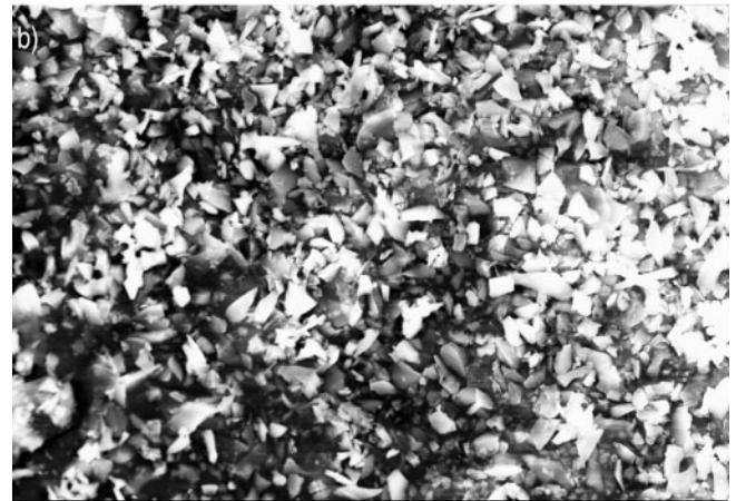
Fig. 4.—a) X-ray diffraction analysis reveals a pattern pointing mainly to amorphous silica, with a tendency to initial, not clearly defined crystallisation processes in the region 20–30 degrees 2\theta . b) Scanning electron microscopy morphological examination shows the presence of irregular particles, similar to broken glass with sharp and pointed angles.
