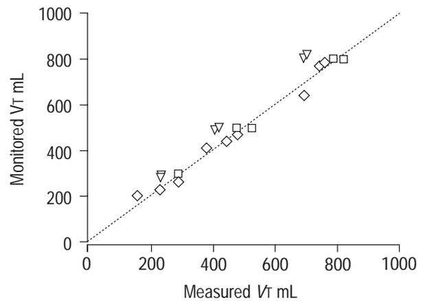
Fig. 3. – Relationship between the observed  $V_T$  and the monitored  $V_T$  for the three ventilators providing  $V_T$  monitoring ( $\square$ : O'nyx plus;  $\diamond$ : Ecole-3-XL;  $\nabla$ : Monnal DCC).
