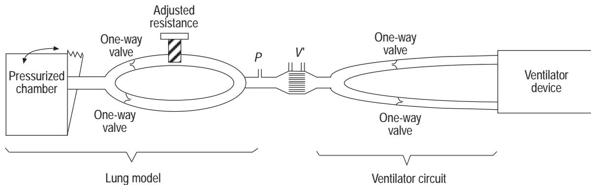
Fig. 1. – The lung model consisted of a pressurized chamber connected to a circuit comprising an expiratory line and an inspiratory line with adjustable resistance, the compliance of the chamber was set at  $30 \text{ mL}\cdot\text{cmH}_2\text{O}^{-1}$ . A pneumotachograph (flow ( $V'$ )) and a differential pressure transducer (pressure ( $P$ )) were inserted between the chamber and the circuit of the lung model.
