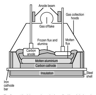
Fig. 2. – Aluminium smelter reduction cell with prebaked anodes (prebake cell) printed with permission [16].
